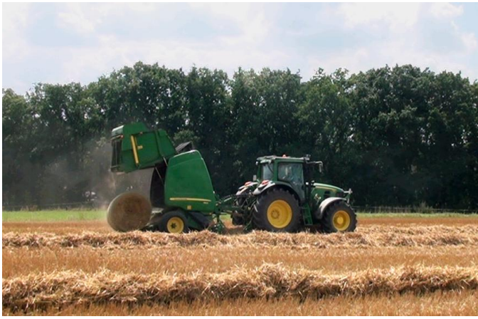
Fig. 1. Application scenario: Tractor with a large round baler following a windrow while collecting the material.
