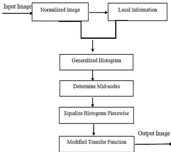
Fig.2. Flow of Histogram Equalization
